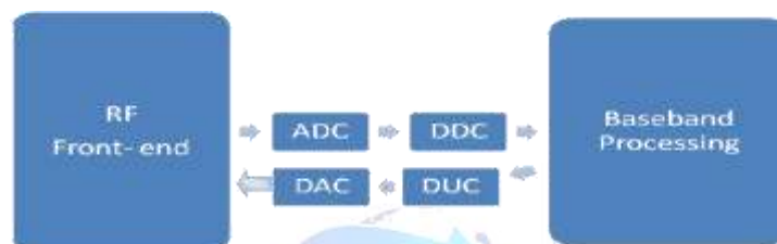
Fig 1: Generic block diagram of SDR
